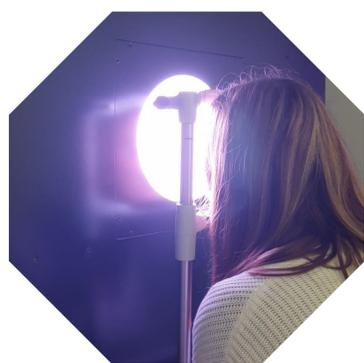
Figure 3. LightBox used in the experimental setup, contains 11 LEDs and forms a Ganzfeld-like illumination
